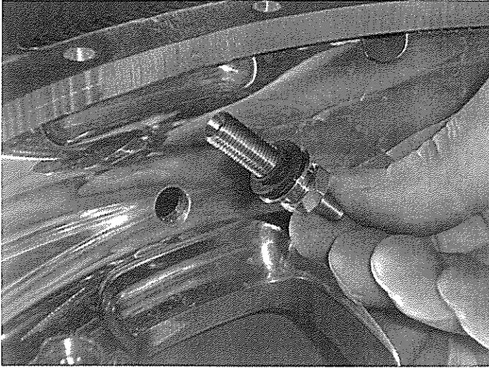
Select the correct grommet for the hole. Insert the stem through the grommet and then through your rim.
