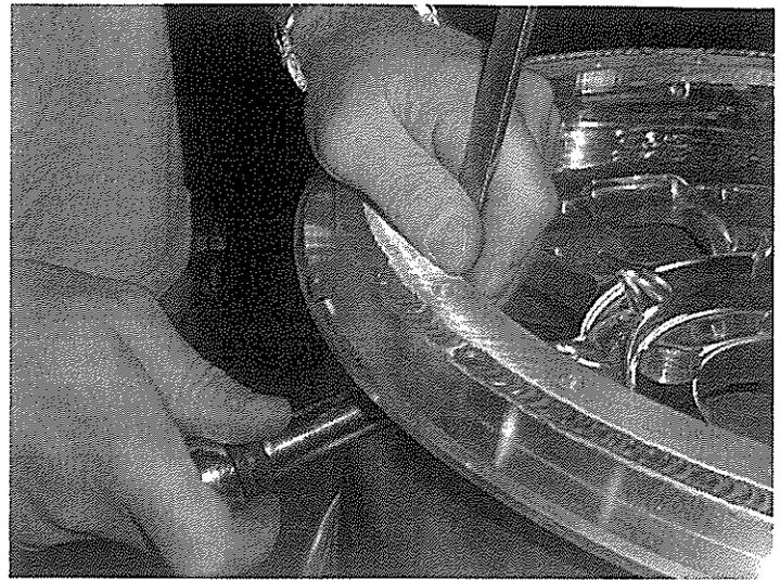
Place the washer on the backside of your rim. Install the Nylock Nut onto the stem. Use the supplied standard jam nut on the external threads-temporarily- to allow you to tighten the Nylock securely, but not so much that the grommet squeezes out
